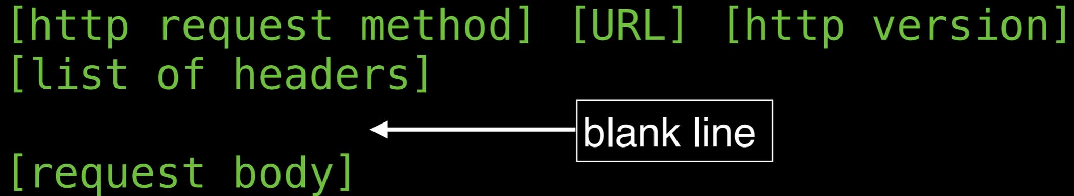
The diagram shows the structure of an HTTP request. It consists of three lines of text in a monospace font, all in green. The first line is "[http request method] [URL] [http version]". The second line is "[list of headers]". The third line is "[request body]". A white arrow points from a box labeled "blank line" to the space between the second and third lines. Another white arrow points from a box labeled "optional" to the "[request body]" line.
